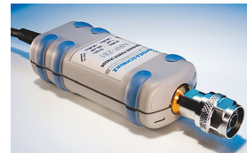
The 50-MHz to 18-GHz NRP-Z81 USB-enabled sensor combines an RF detector with analog- and digital-signal-processing capability to add full power-meter functionality to a PC.
